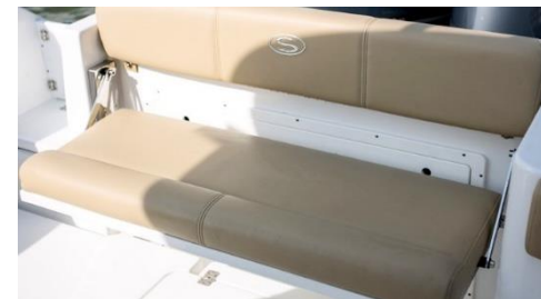
The rear seat easily detaches to allow easy access to the bilge area at the stern.
