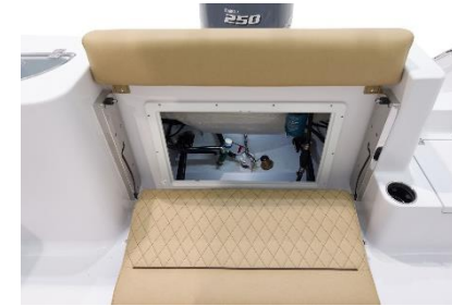
The rear seat easily detaches to allow easy access to the bilge area at the stern.
