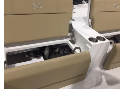
The rear seat easily opens to allow easy access to the bilge area at the stern.
