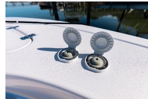
BOW CONTROLS FOR ANCHOR
