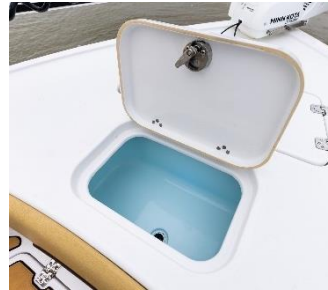
Bow Livewell (w/ overflow, fill valve, and drain)
