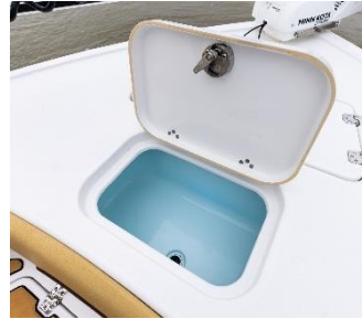
Bow Livewell (with overflow, fill valve, and drain)
