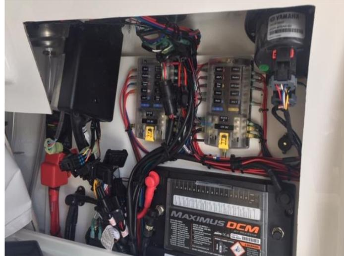
The system communicates through NMEA2000 to your Garmin MFD to add a screen that shows all of your 12v switches, doing away with the need to have physical toggle switches on the dash. You are able to customize the look and feel of the switches as well as create presets and modes with your favorite combination of lights. This type of flexibility is just not possible without digital switching.
