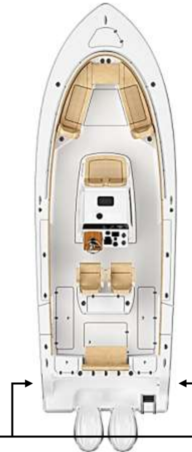
The rear seat easily detaches to allow easy access to the bilge area at the stern.
