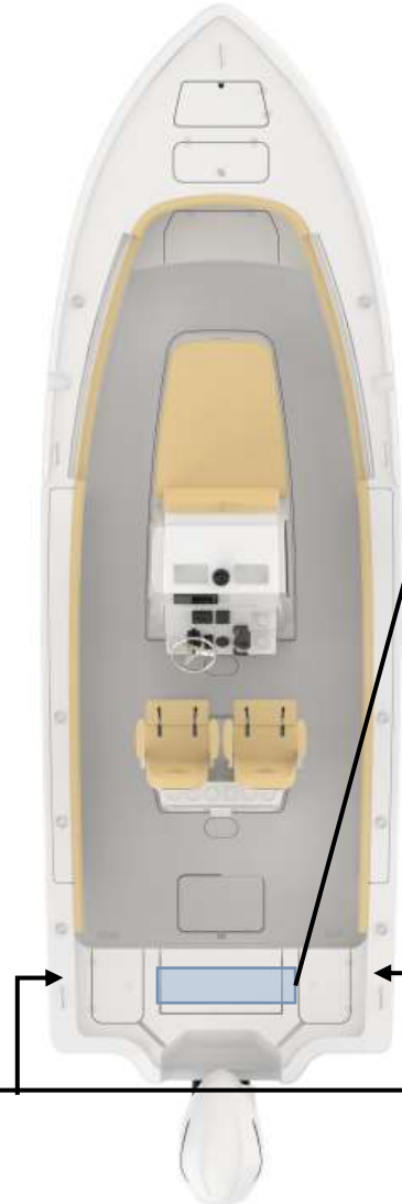
The rear seat easily opens to allow easy access to the bilge area at the stern.
