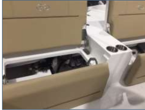
The rear seat easily opens to allow easy access to the bilge area at the stern.
