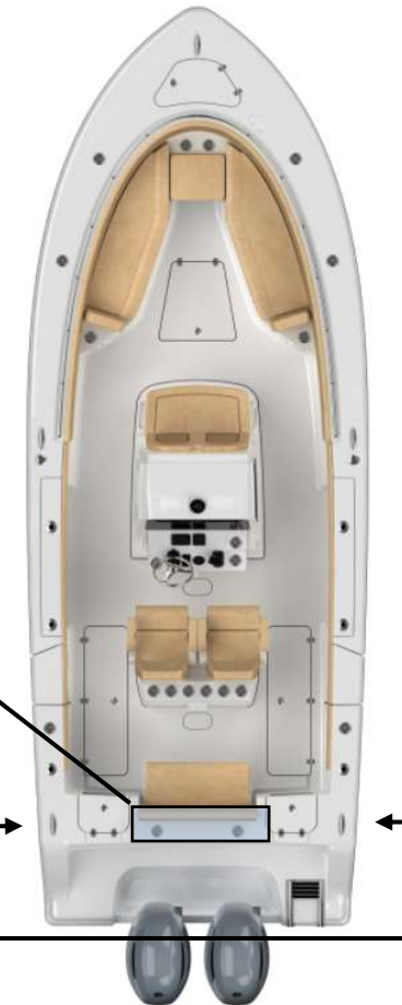
The rear seat easily opens to allow easy access to the bilge area at the stern.
