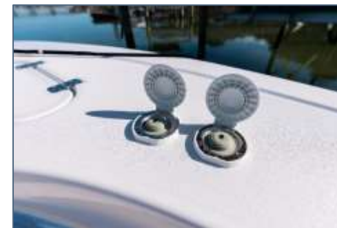
BOW CONTROLS FOR ANCHOR
