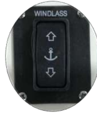
CONTROL ON THE HELM FOR THE ANCHOR
