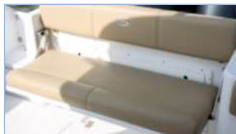
The rear seat easily detaches to allow easy access to the bilge area at the stern.
