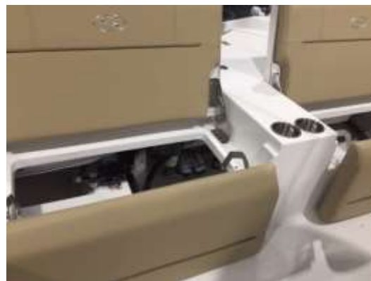
The rear seat easily opens to allow easy access to the bilge area at the stern.
