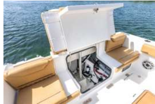
The rear seat easily opens to allow easy access to the bilge area at the stern.
