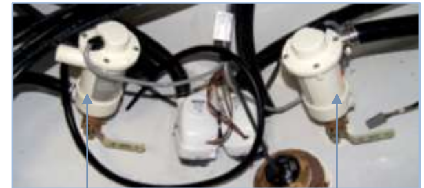
Pumps To Fill Valves
