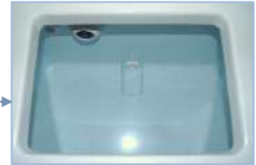
Console Seat Livewell (with overflow, fill valve, and drain)
