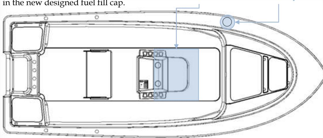
The fuel tank can be accessed through the panel forward of the helm, pictured above. **Pease note that this is an access point. Should you choose to store non-constrained items here while the boat is in transit, they may shift to an inaccessible area under the deck of the boat. We recommend using the provided removable bag to hold items in this space.**
