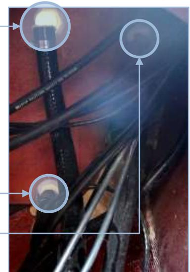
Pictured above is the plumbing system for the rear livewell. The pump is connected with a hose to the fill valve located at the top of the livewell tank. The overflow drain and drain hoses meet in a "Y" joint to drain out the thru hull at the transom.
