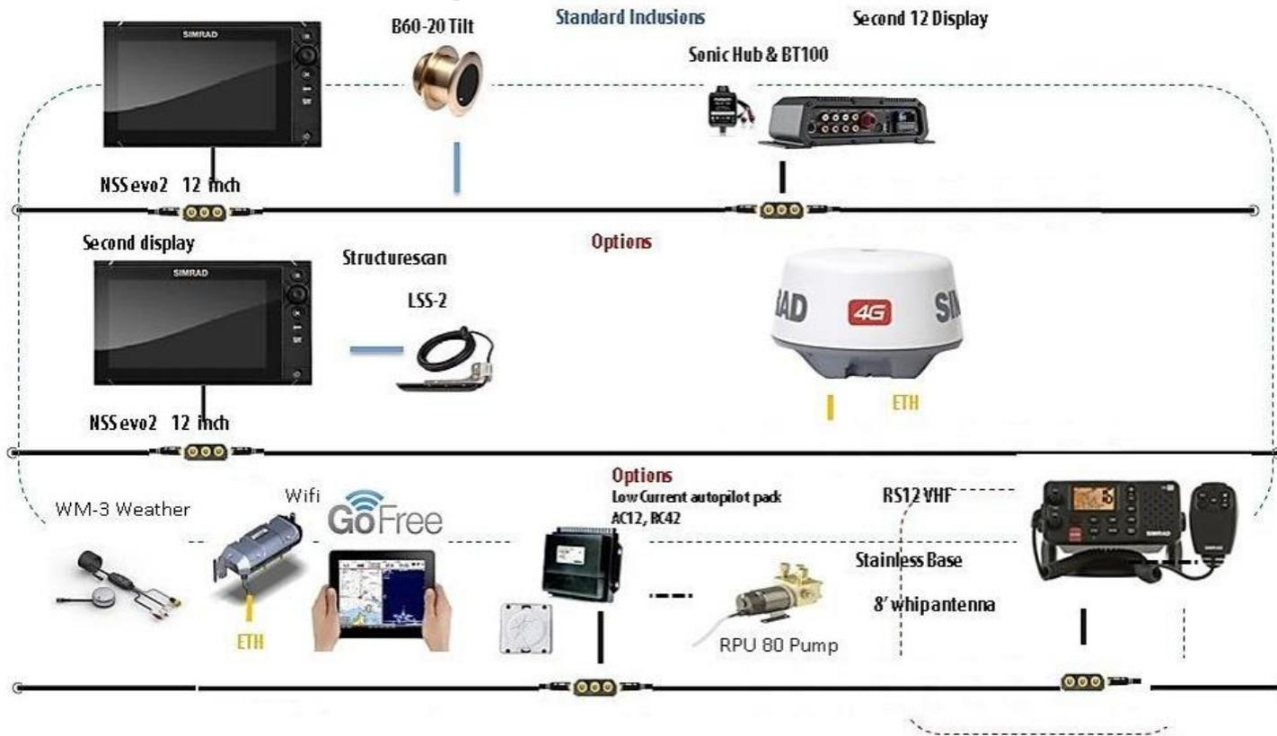
The Sportsman Open 252 includes a 12" Simrad unit as a standard feature. The transducer is located on the hull bottom at the stern of the boat. The SonicHub system is another standard feature of the Open 252 and is located on the inside wall of the console. The SonicHub system is controlled through the Simrad unit.
