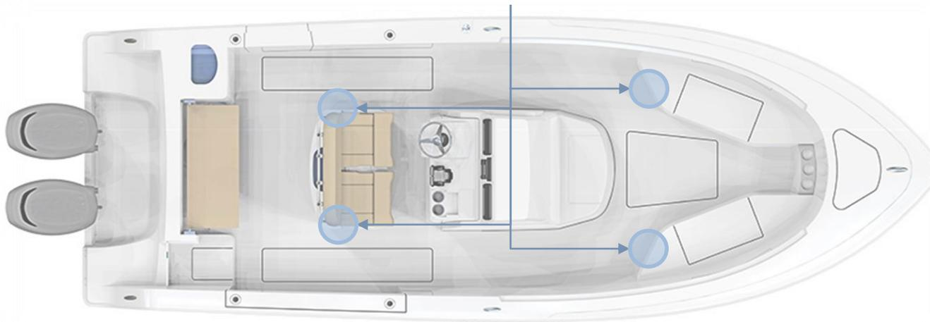
The aft pair of speakers (the left two speakers in the figure to the left) are located on the T-Top underside.
