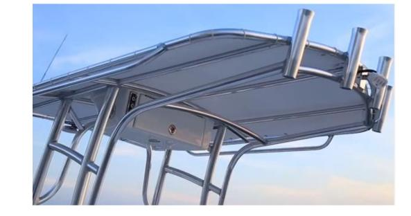
Deluxe T-Top option. Comes with a E box for an extra storage space. The T-Top switch turns on the blue courtesy light. The SPREADER switch operates the front and back spreader light.
