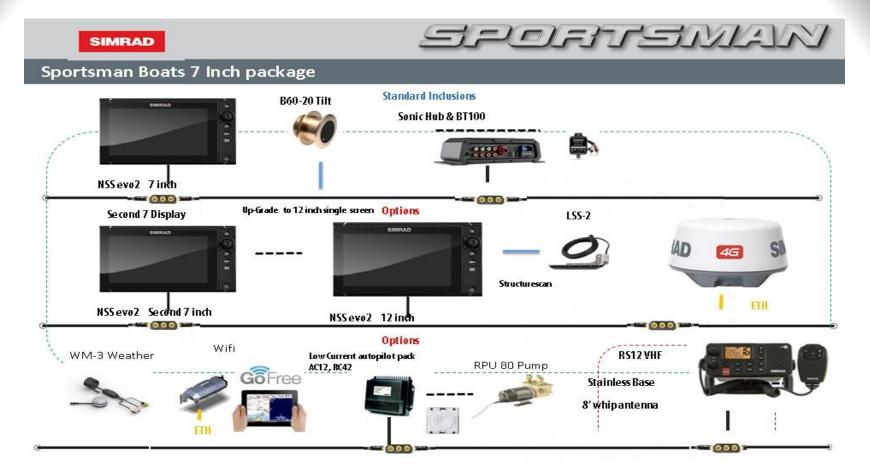
Your Sportsman 232 Open comes with a Standard 7" Simard Unit. The Transducer is located on the hull bottom at the stern of your boat. The Sonic Hub is also standard on your 232 Open, and is controlled through your Simrad display unit. The Sonic Hub is located inside your console.
