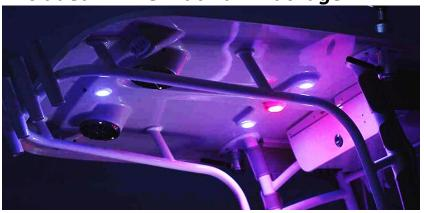
Fiberglass Top option comes with the Platinum package. The T-Top switch turns on the 3 blue courtesy lights. The SPREADER switch operates the 2 back spreader lights and the front spreader light. The switch on the map light may be turned one way for a red or the other way for a white light.
