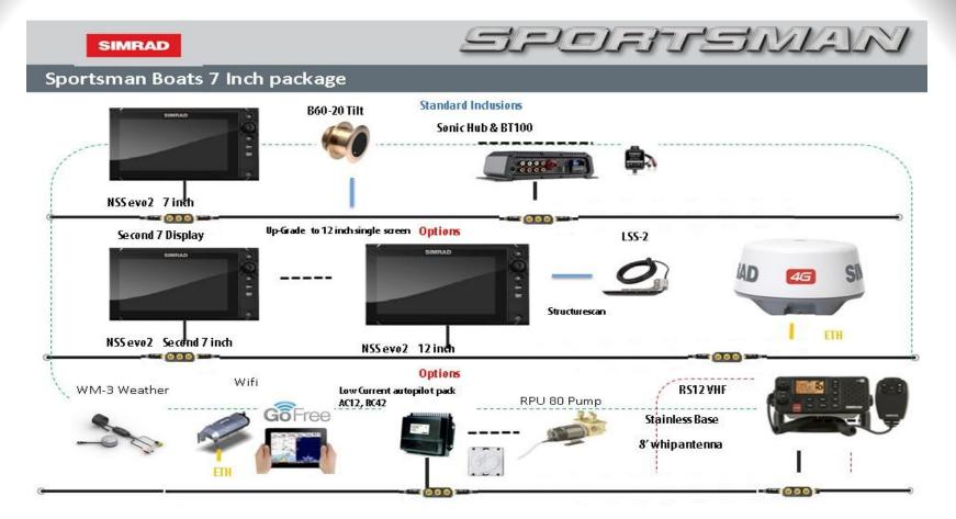
Your Sportsman 212 Open comes with a Standard 7" Simard Unit. The Transducer is located on the hull bottom at the stern of your boat. The Sonic Hub is also standard on your 212 Open, and is controlled through your Simrad display unit. The Sonic Hub is located inside your console.
