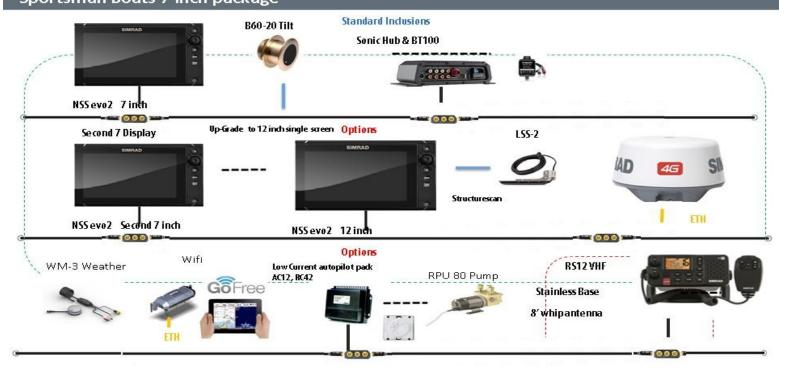
Your Sportsman 211 Heritage comes with a Standard 7" Simard Unit. The Transducer is located on the hull bottom at the stern of your boat. The Sonic Hub is also standard on your 211 Heritage, and is controlled through your Simrad display unit. The Sonic Hub is located inside your console.
