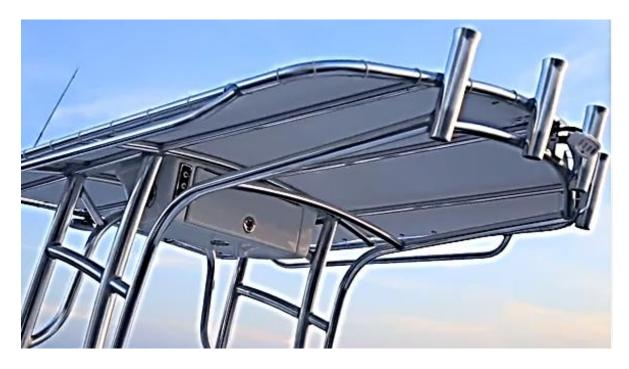
Deluxe Soft Top option comes with the Sport package. The T-Top switch turns on the blue courtesy light. The SPREADER switch operates the front and back spreader light.
